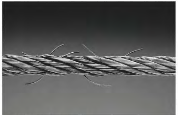
Cable With Broken Wires
